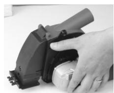
3) Fix the inner flange, then put the first blade(picture c)
