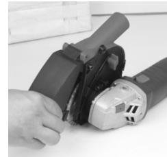
2) Loosen the screw on the left side by the accessory inner hexagon spanner.(picture b)
